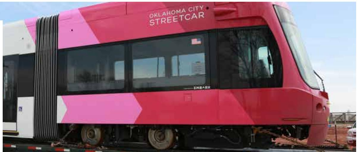
Each streetcar must have at least 310 miles of testing before certification to carry passengers, and streetcar testing will be ongoing until the scheduled start of service late this year. Testing will begin along the Downtown Loop when construction is completed on that track in late summer.
